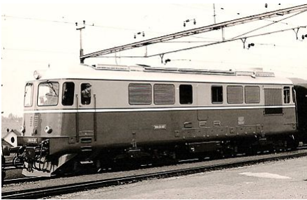
First Romanian Railways CFR Class 60 locomotive built in Switzerland
