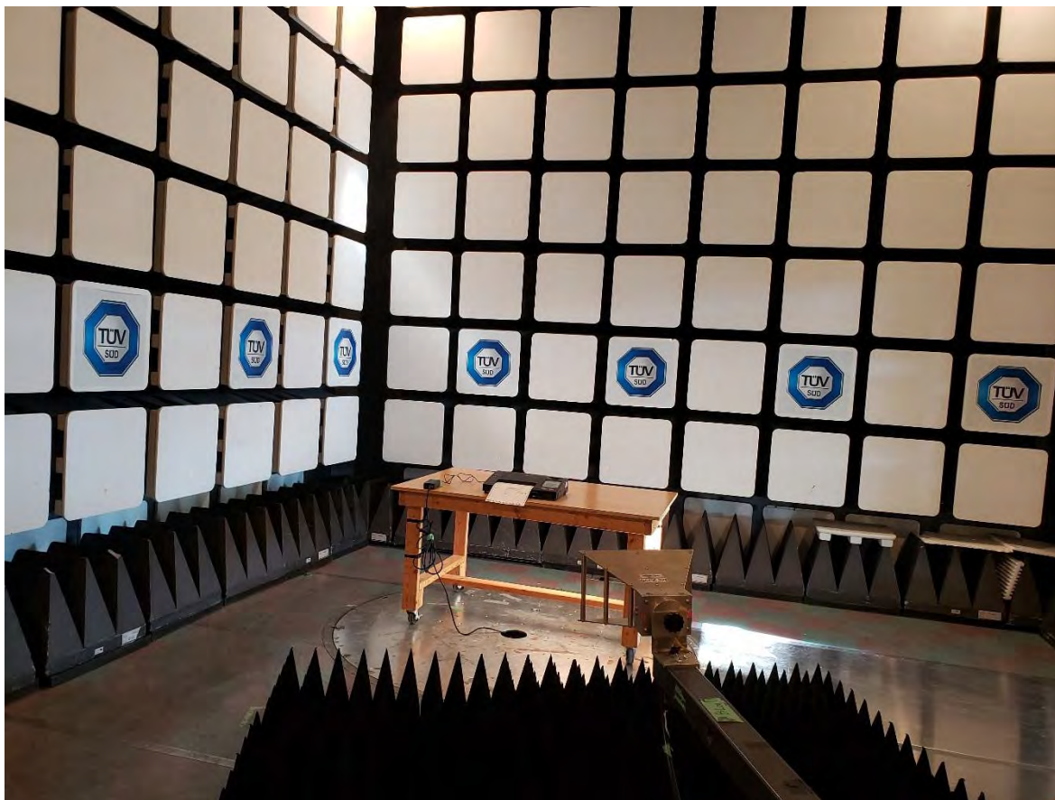
Figure 8 – Radiated Emissions Setup – Photo 2 1GHz – 6GHz
