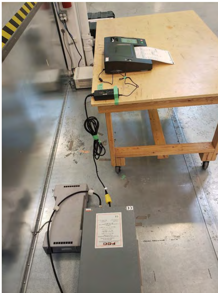
Figure 6 – Power Line Conducted Emissions Setup – Photo 2
