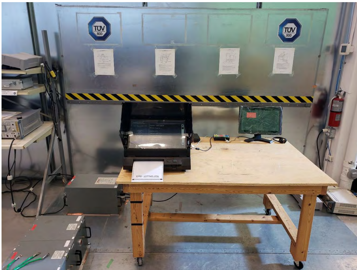
Figure 8 – Power Line Conducted Emissions Setup – Photo 2
