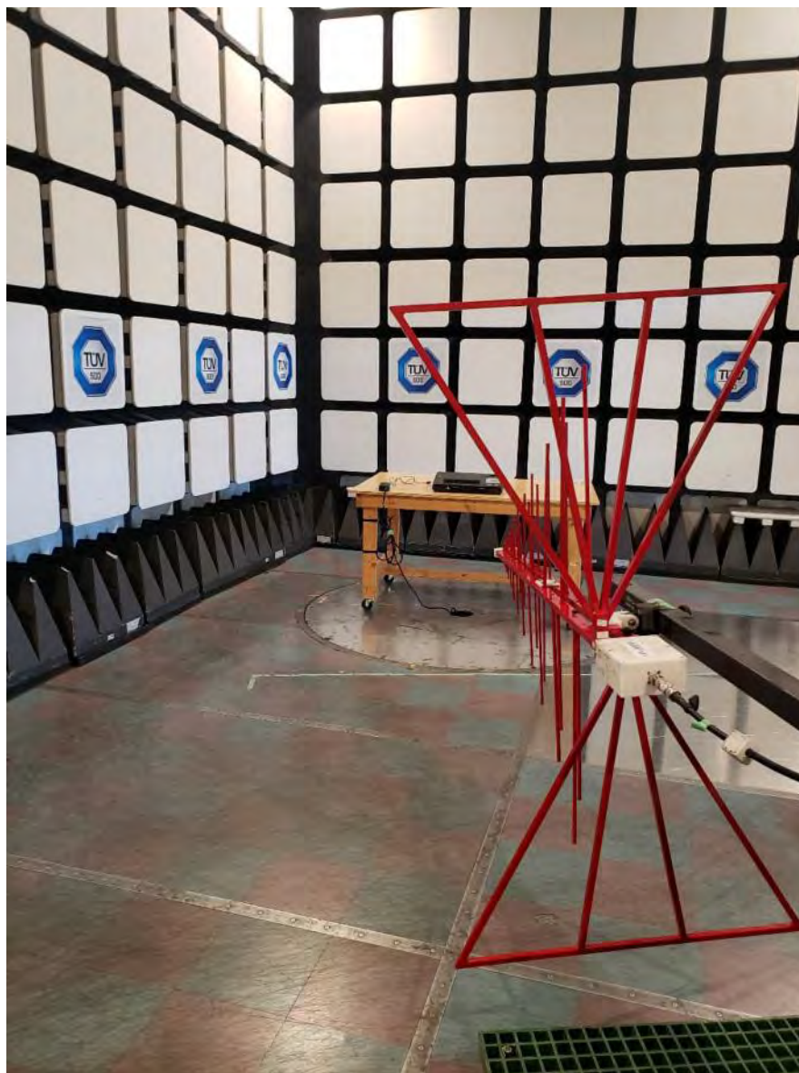
Figure 7 – Radiated Emissions Setup – Photo 1 30MHz – 1GHz
