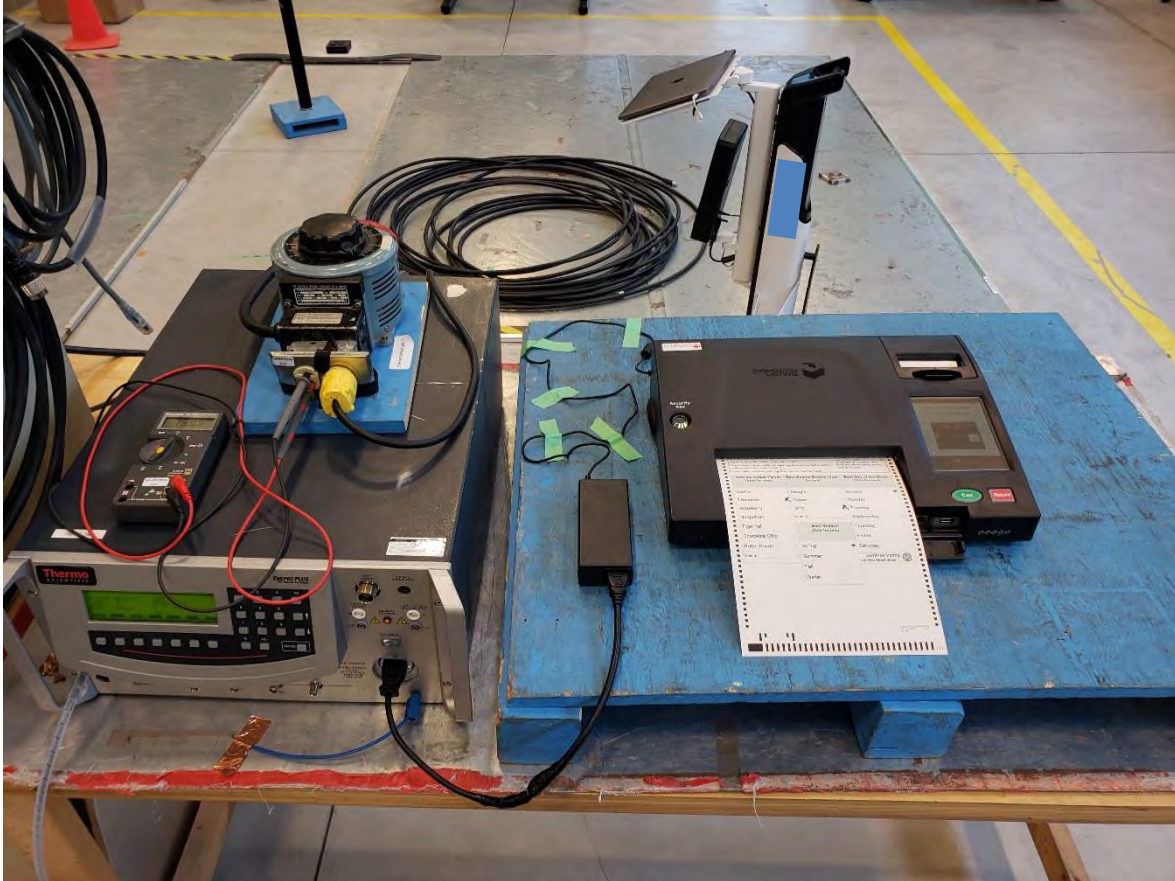
Figure 9 – Electrical Power Disturbance – Surges of \pm 15\% Line Variations
