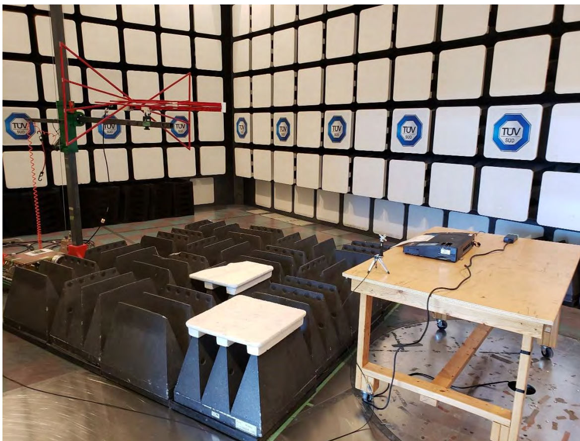
Figure 15 – Electromagnetic Susceptibility Setup – Photo 2
