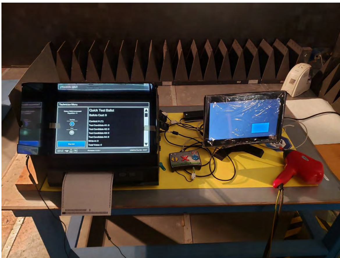
Figure 13 – Electrostatic Disruption Setup
