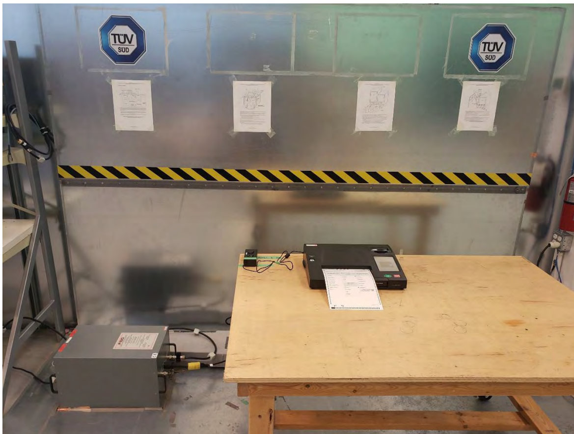
Figure 5 – Power Line Conducted Emissions Setup – Photo 1
