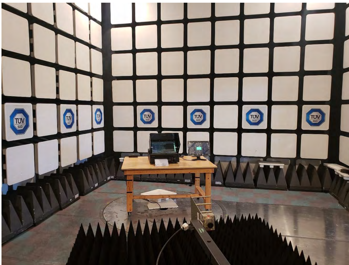
Figure 10 – Radiated Emissions Setup – Photo 2 1GHz – 6GHz
