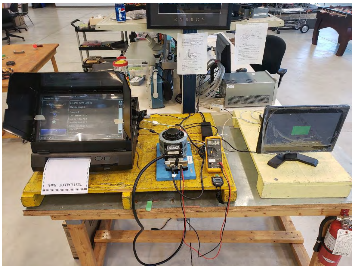
Figure 12 – Electrical Power Disturbance – power increase & reduction
