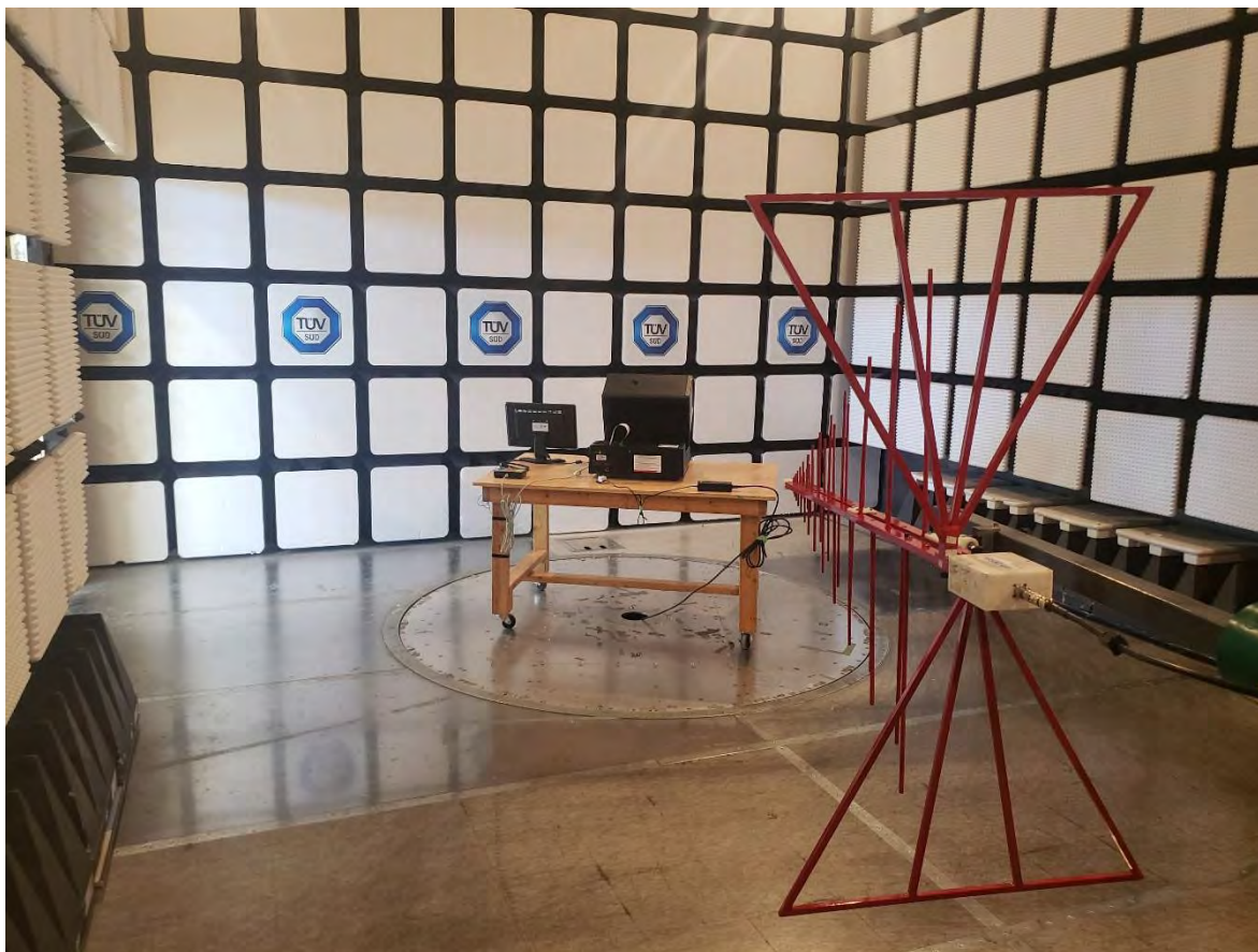
Figure 9 – Radiated Emissions Setup – Photo 1 30MHz – 1GHz
