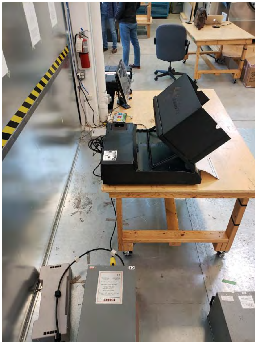
Figure 7 – Power Line Conducted Emissions Setup – Photo 1
