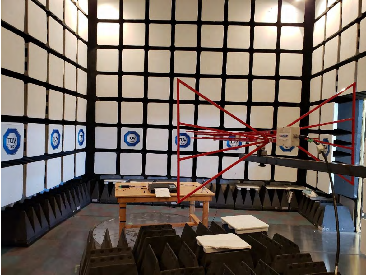
Figure 14 – Electromagnetic Susceptibility Setup – Photo 1
