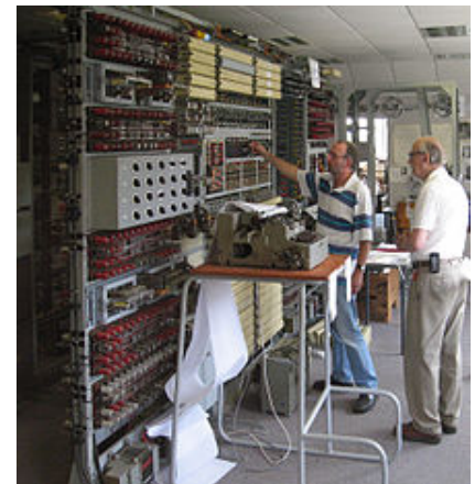
In 1994, a team led by Tony Sale (right) began a reconstruction of a Colossus at Bletchley Park. Here, in 2006, Sale supervises the breaking of an enciphered message with the completed machine.
