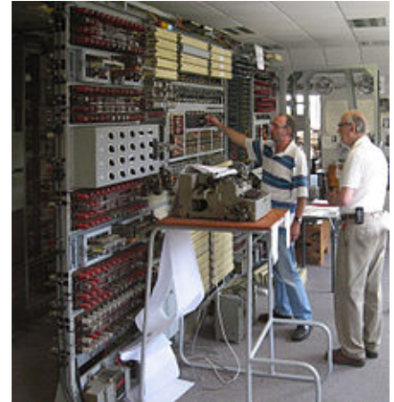
A team led by Tony Sale (right) reconstructed a Colossus Mark II at Bletchley Park. Here, in 2006, Sale supervises the breaking of an enciphered message with the completed machine.
