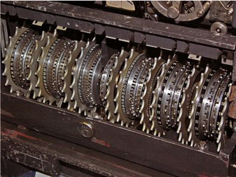
The Lorenz SZ machines had 12 wheels, each with a different number of cams (or "pins").
