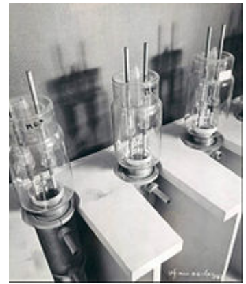
High frequency tubes in the tube room. They were used for the NBC television transmitter, 1936. NBC kept 220 tubes in reserve for their transmitter.
