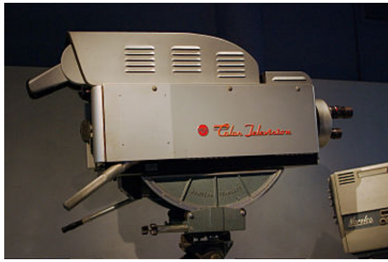
1954 RCA TK-41C dolly-mounted color broadcast camera
