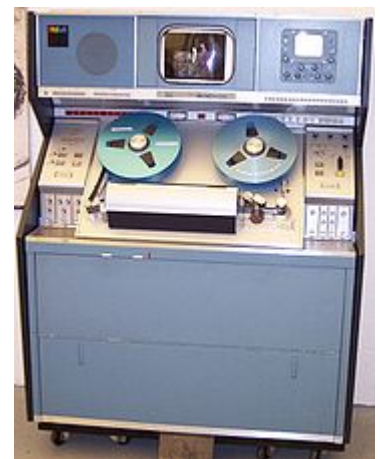
RCA Television Quad head 2" color recorder/reproducer used at broadcast studios in the late-1960s, '70s and early-'80s. [39]
