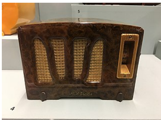
RCA Model RC-350-A (1938) radio, made of Catalin and Bakelite
