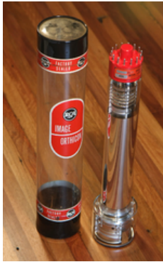
1970s-era RCA Radiotron Image Orthicon TV Camera Tube
