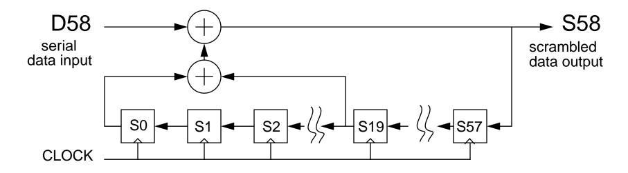
The serial form of the scrambler is shown here for bit ordering purposes. Parallel implementations could also be used. For details see:
