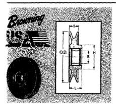
For "4L", "A", "5L" and "B" belts Cast-iron construction Needle bearings
