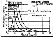
Theoretical deflection of the piston rods in their extended position may be calculated by using the preceding formulas for either a transverse or torsional load.
