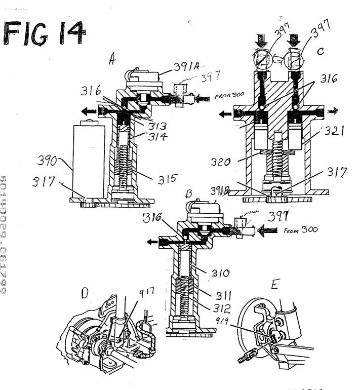
FLOW ALTERATIONS FOR MODULATOR SEIYSORS. AND WHEEL VALUE
