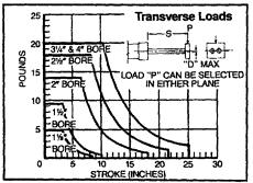
Transverse or torsional loads placed on the cylinder will cause some deflection of the piston rods. Excessive deflection will adversely affect cylinder life and should be considered at the time of initial application design.
