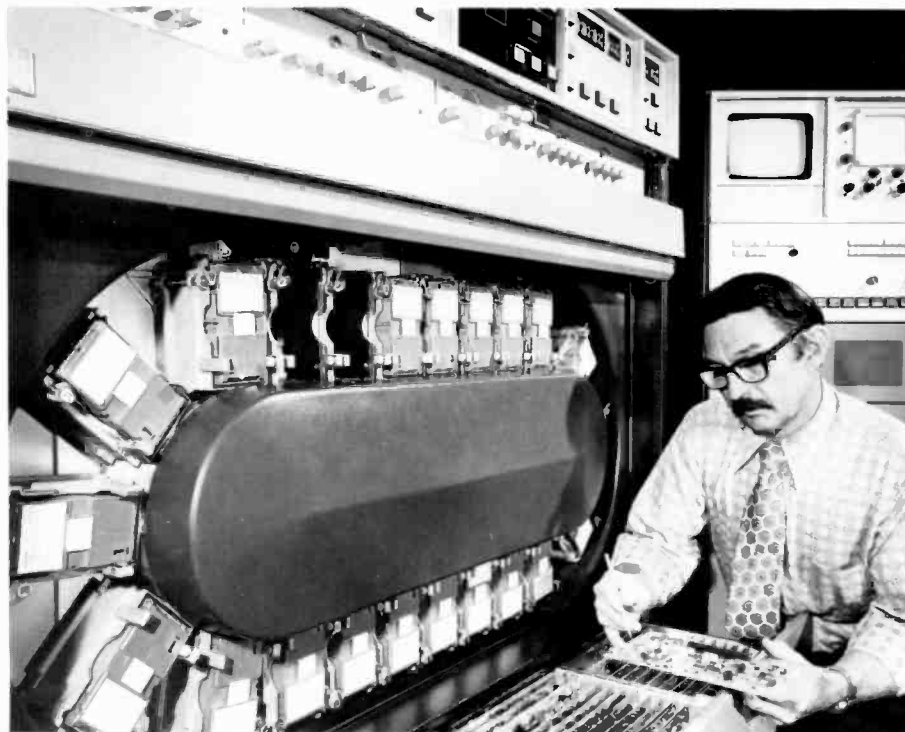
16. TCR-100 Video Tape Cartridge Recorder/Player makes automated station breaks possible.
