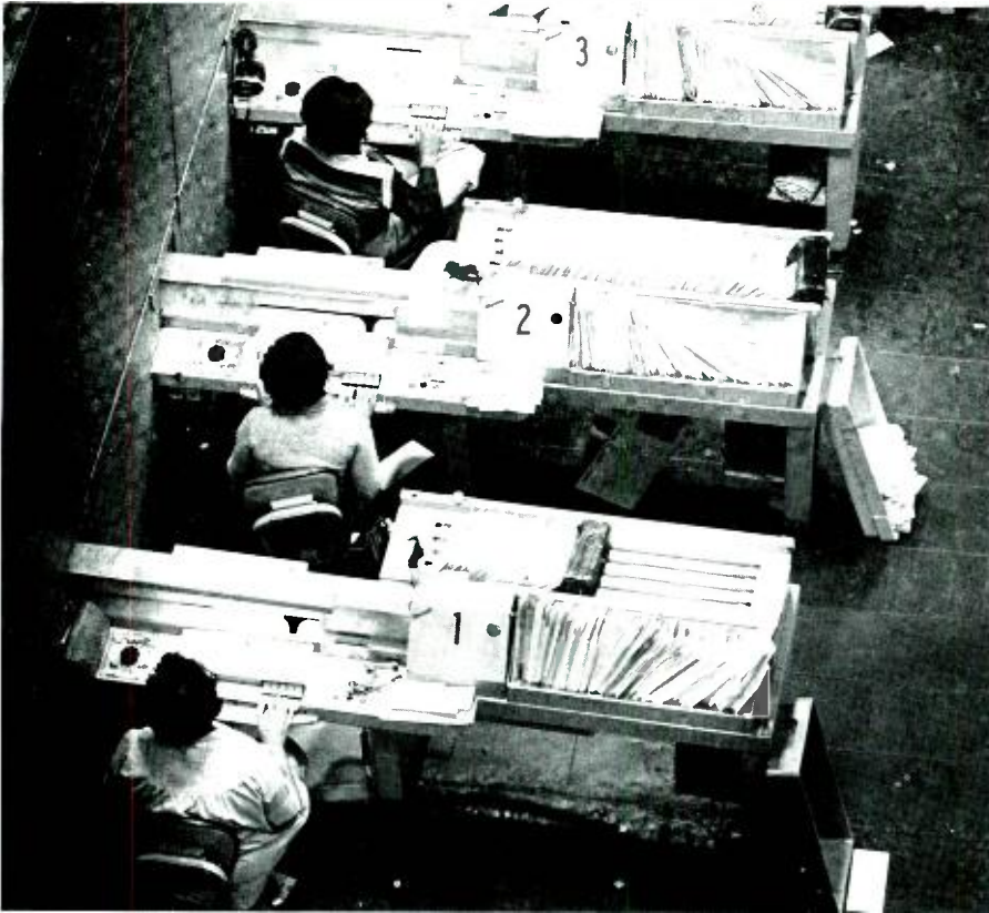
Postal Sectional Centers and Area Distribution Centers contain letter sorting machines. In these machines, unsorted letters are mechanically moved to a position in front of an operator who keyboards address data. This keyed data causes the letter to be moved to a correct output sort bin. Re-sort at several locations is typical for a letter traversing the country.
