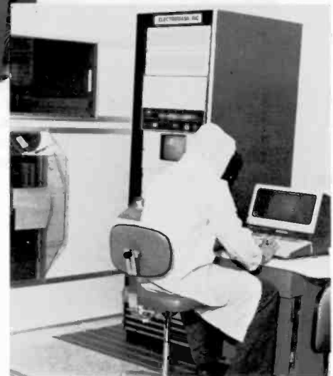
6. Mask defects will print on wafers. If a perfect mask never touches the wafers, better yields can be expected. This Perkin-Elmer aligner uses scanning-projection mirror optics that allow deep-ultraviolet exposures for better resolution.
