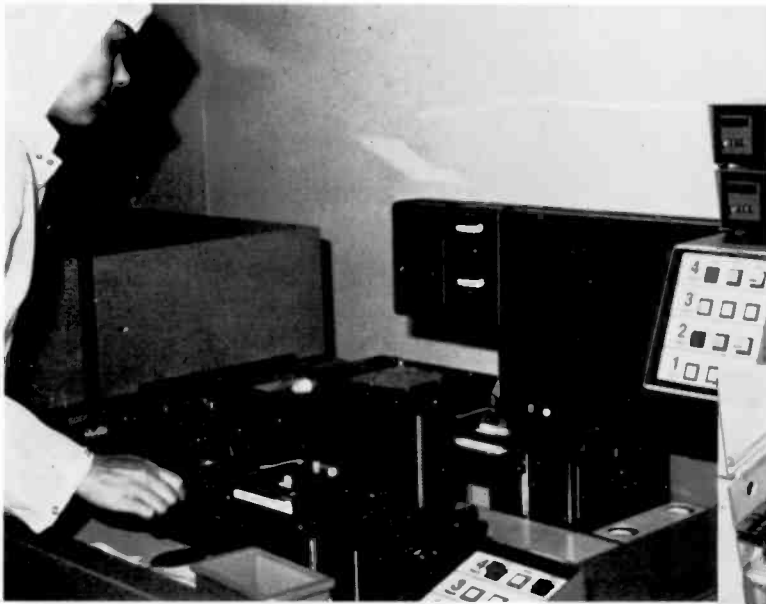
3. Patterning precision is achieved by photoengraving. The silicon wafer is coated with an ultraviolet-sensitive photoresist. This process is highly automated.
