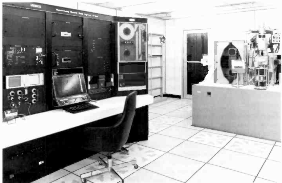
Fig. 1. MEBES mask and reticle drawing facility in a specially controlled clean room environment. The actual drawing equipment is shown on right and the computer console control is shown on left.
