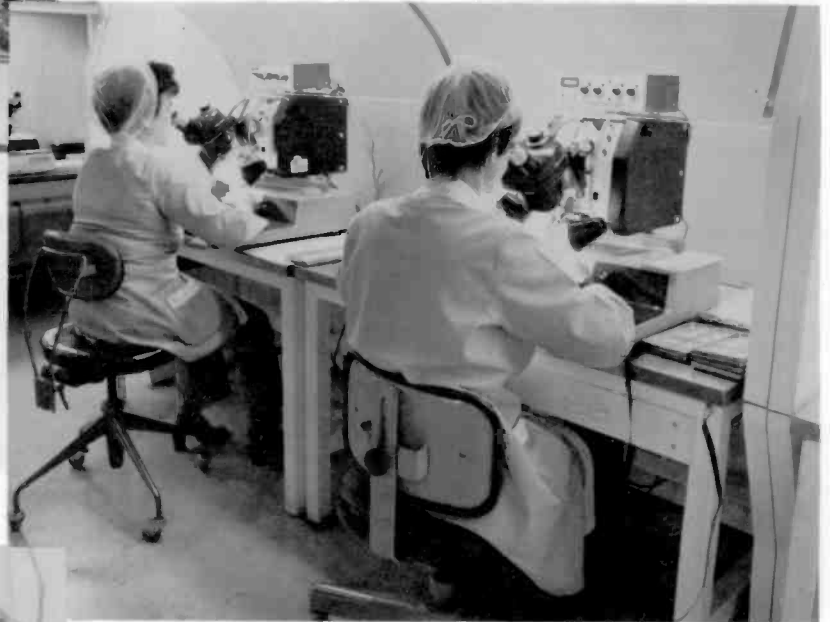
17. Dicing the wafer and mounting the pellets onto headers is done next. Then wires are bonded between the integrated circuit chips and the package leads. This is by far the most labor-sensitive area of integrated circuit fabrication. For SSTC integrated circuits, visual inspection procedures are rigorous.
