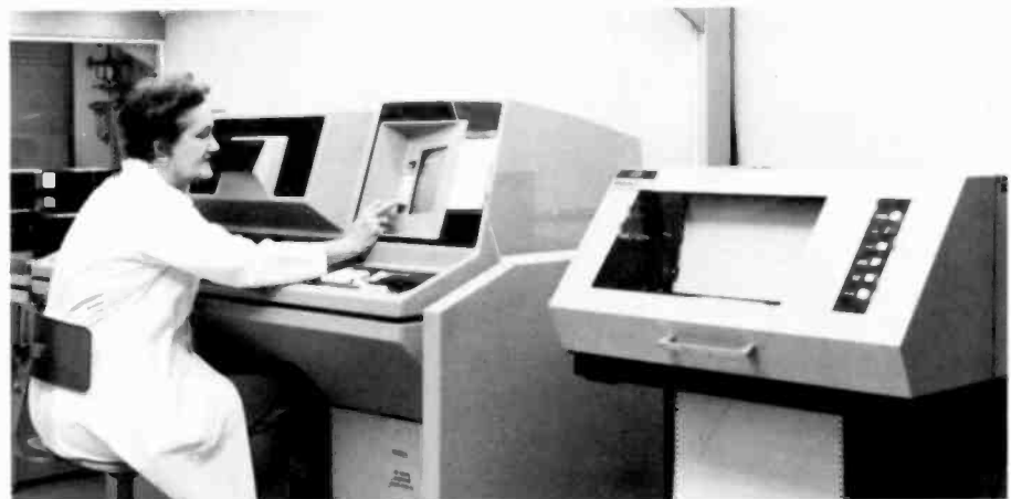
Fig. 2. KLA-100 automatic 100 percent mask inspection machine. This machine has a defect detection capability down to 2\ \mu\text{m} and produces a hard copy map of all defects detected. It is tied directly to a laser chrome defect removal machine (see Fig. 3) and common software and data is shared between equipment.
