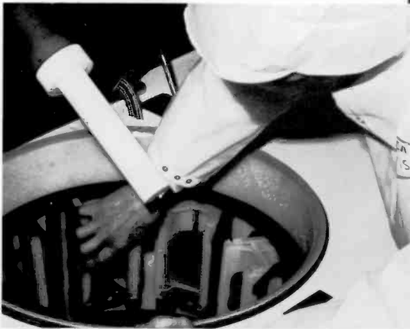
10. This FSI spray-etch station looks like a washing machine. It allows 150 four-inch wafers to be cleaned, etched, rinsed and dried in one operation. Again, a computer terminal controls the operation and prevents incompatible chemicals from being sprayed together.
