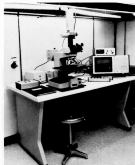
Fig. 6. An ultra precision ITP, digital, microdensitometer line edge sensing machine used to measure critical dimensions down to 1½ \mu m to an accuracy of \pm 2 \mu inches.
