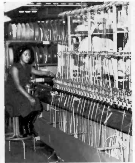
Fig. 5 Sequencer puts components onto reels in the proper sequence for the variable-center insertion equipment shown in Fig. 4. Also computer-driven, this machine cuts the components from their original reels and reels them again in the proper sequence.
