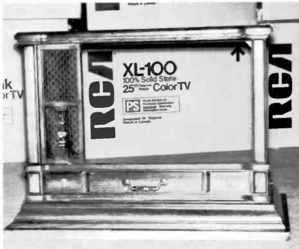
Fig. 13 Ready to go. The fully finished wood cabinet is now ready for packing and shipping to RCA's final assembly plant at Bloomington, Ind.
