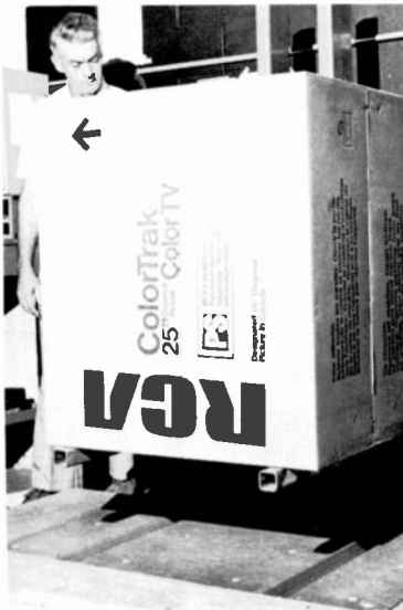
Fig. 13 (top left) Shock hazard test on a typical 25-inch set.
