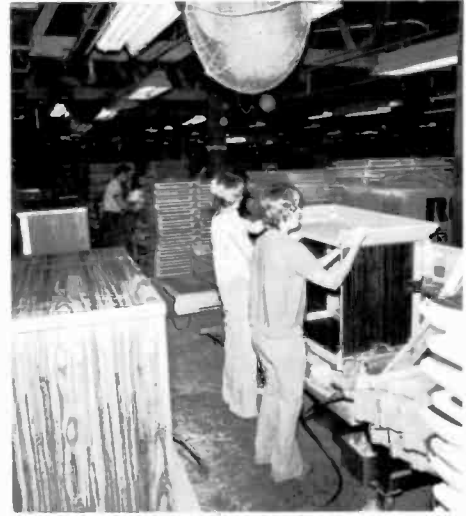
Fig. 8 The layup operation sees all the detail parts and assemblies come together. A furniture-type cabinet requires proper gluing and doweling before automatic nailers and screwdrivers are used to hold the multiple assemblies together.
