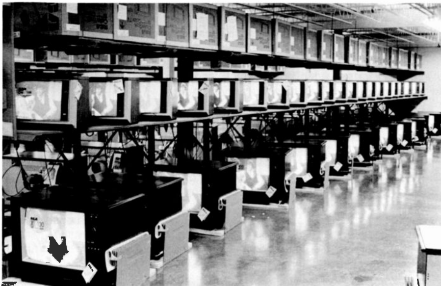
Fig. 17 Long-term life testing. There are always 1000 sets undergoing this performance evaluation at elevated line voltage and ambient temperature.
