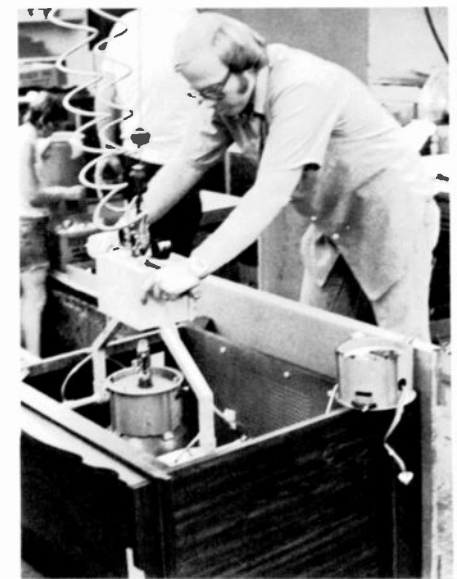
Fig. 7 (right) Yoke-assembly press. The yoke is being assembled to the tube at the left. Extremely critical assembly controls are necessary to avoid picture-tube neck damage during yoke positioning and to make sure that the yoke adheres to the picture-tube bell properly.
