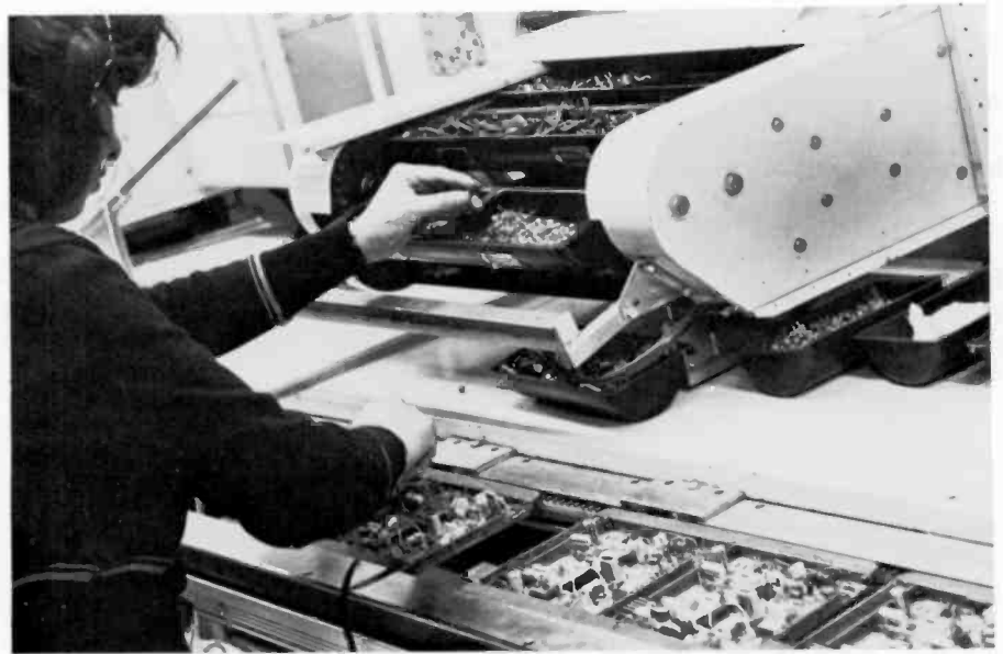
Fig. 6 In-line conveyor brings components to operator for manual insertion on boards that move along conveyor in foreground. Ground strap on operator's right arm protects ICs from static discharges.
