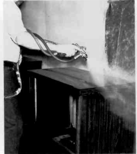
Fig. 11 Lacquer coat gives the cabinet a glossy appearance. The "waterfall" at right keeps fumes away from operators.
