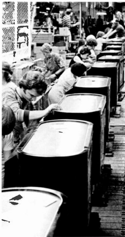
Fig. 4 Typical production line for color tv receivers. The continuously moving wooden slat conveyor carries the work-in-process instrument past the operators, while an overhead belt conveyor (not shown) transports the empty cartons to the end of the line. The monorail conveyor in the left background is delivering chassis to their required assembly position. Manufacturing engineers must design processes around the existing lines.
