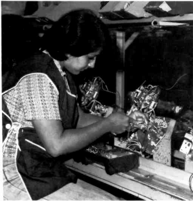
Fig. 9 Deflection modules are assembled on a chain conveyor; most of the assembly work consists of interconnecting wires by crimping, soldering, and wire-wrapping.
