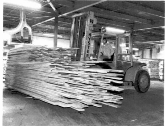
Fig. 1 In about three hours, this rough lumber will be all television cabinets and sawdust. The rough lumber arrives at RCA as boards with thicknesses 1" to 2", lengths at 10-12', and average widths of 7". Air- and oven-drying has reduced the moisture content to 6-8%.
