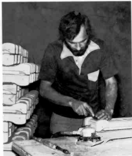
Fig. 9 Cleaning up and sanding is an operation that cannot be done by machine. The glue, wood chips, and some wood-filling material must be removed, and then the wood must be sanded, before the cabinet gets its finishing coats. This "white wood preparation" is very important to the finished quality of the cabinet.
