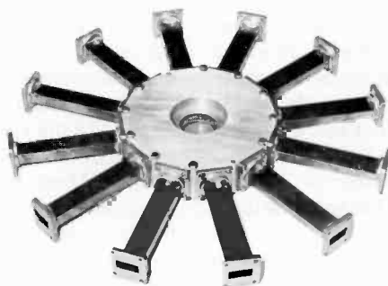
Fig. 14 Low-loss dual-mode radial waveguide power divider for feeding a circular cylindrical array antenna.
