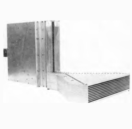
Fig. 11 Dual-mode sectoral horn power divider for a single-plane-scanned, low-sidelobe phased array. The low-loss "optical divider" properties of this horn make it attractive for millimeter-wave array applications.
