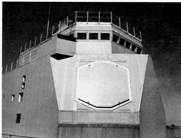
Fig. 3 Modern phased-array radar , the AN/SPY-1A, is used in air-defense system on Navy ships, four antenna faces per ship. This face is on the developmental site at Missile and Surface Radar, Moorestown.
