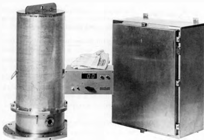
Fig. 3 System has three major components—microwave electronics/antenna enclosure (left) and signal-processing enclosure (right), which are installed on the furnace top, and display enclosure, which goes in furnace control room.
