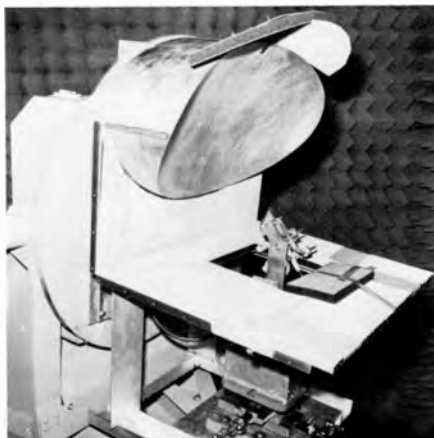
Fig. 6 One-tenth scale model verified low-sidelobe responses predicted by computer simulation. Operating frequency covers 31 GHz to 36 GHz. Test feed horns were designed to provide either horizontal or vertical linear polarization.
