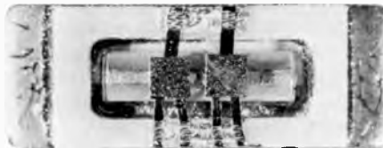
Fig. 2 "Flipped" device mounted on a gold-plated copper carrier. This technique provides good heatsinking and low source inductance.
