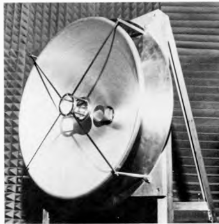
Fig. 10 A new wideband multimode monopulse feed for a small Cassegrain antenna. The new mode-generating technique has doubled bandwidth capabilities.
