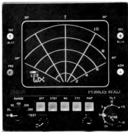
Fig. 7 High-resolution dot pattern for range azimuth markers is difficult to produce on a 525-line tv raster. Special LSI circuit makes the dots appear as smooth lines.
