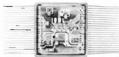
Fig. 2a Higher-frequency digital operation is possible with hybrid circuits than with packaged components on pc boards. Thick-film hybrid here is capable of 640-MHz operation. Package is 1.25" square.
