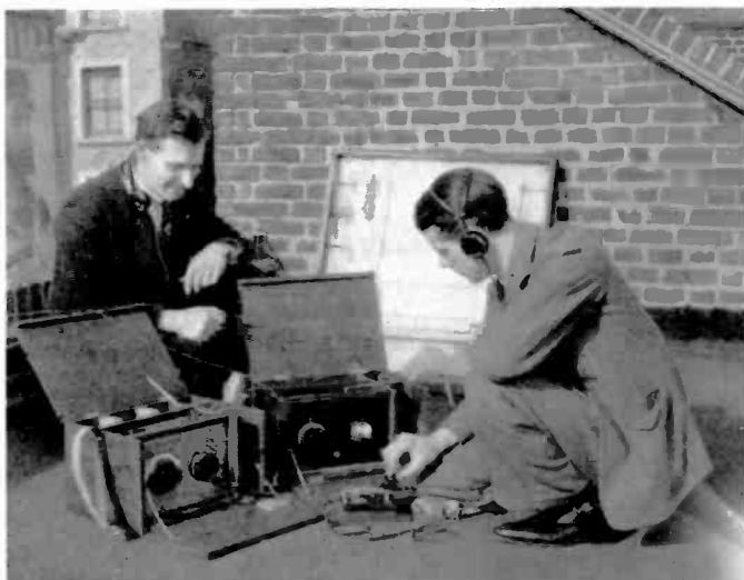
The battery operated 3.5 Mc/s and 7 Mc/s transmitter and receiver used by the Oxford University Arctic Expedition 1933. The transmitter employed a tuned-plate fixed-grid high-capacity circuit and produced an output of three watts. Loomes' Radio (Reg. Loomes, G6RL, left, Eddie Read, G6US, right) were the manufacturers.
