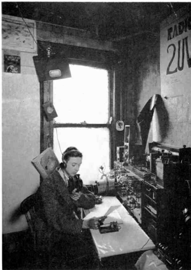
W. E. F. Corsham, 2UV, operating the equipment he used for experimental transmissions between his station in North West London and the station of R. D. Spence, 2JZ, in Huntly, Aberdeenshire in July 1922. The wavelength used was 180 metres.
