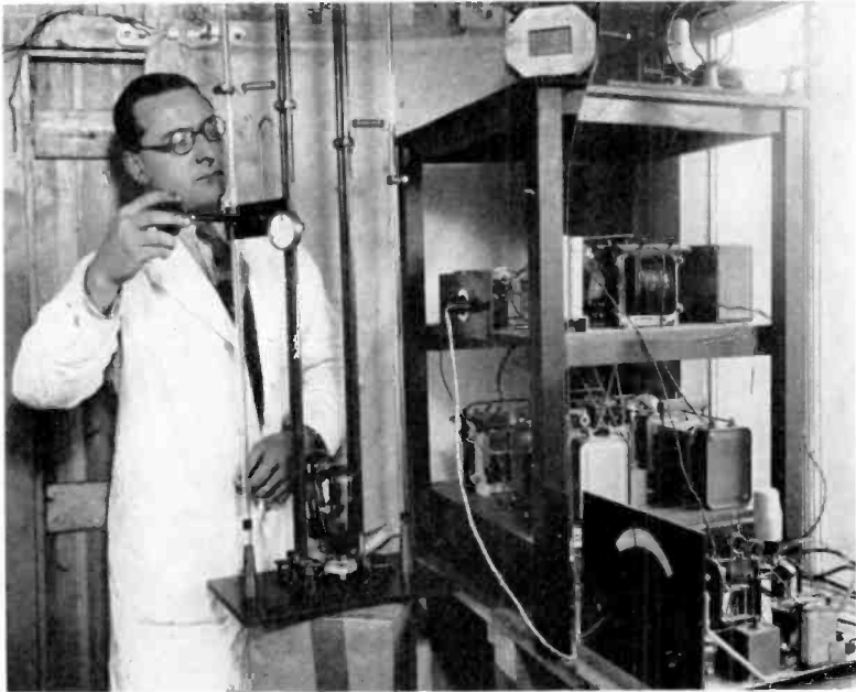
George Brown, G5BJ, adjusting an experimental 58 Mc/s transmitter which operated during 1935, from the works of Stratton & Co. Ltd., Birmingham. A pair of Mullard TZ 0/25 valves in push-pull produced an input power of 50 watts. Signals were well received up to distances of 20 miles.
