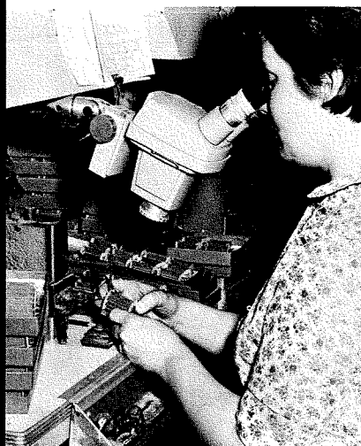
Fig. 4—Grid lineup performed by experienced operator.
