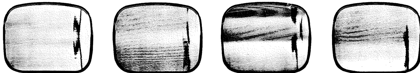
Fig. 6—Typical snivet interference on picture-tube raster.
