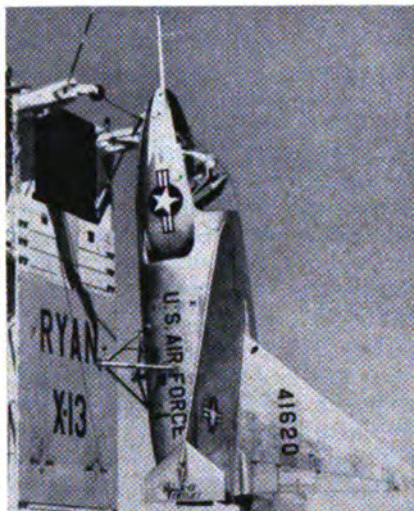
The Air Force's Ryan X-13 Vertijet, pictured here, is capable of taking off in a vertical attitude and quickly switching to high speed horizontal flight.
