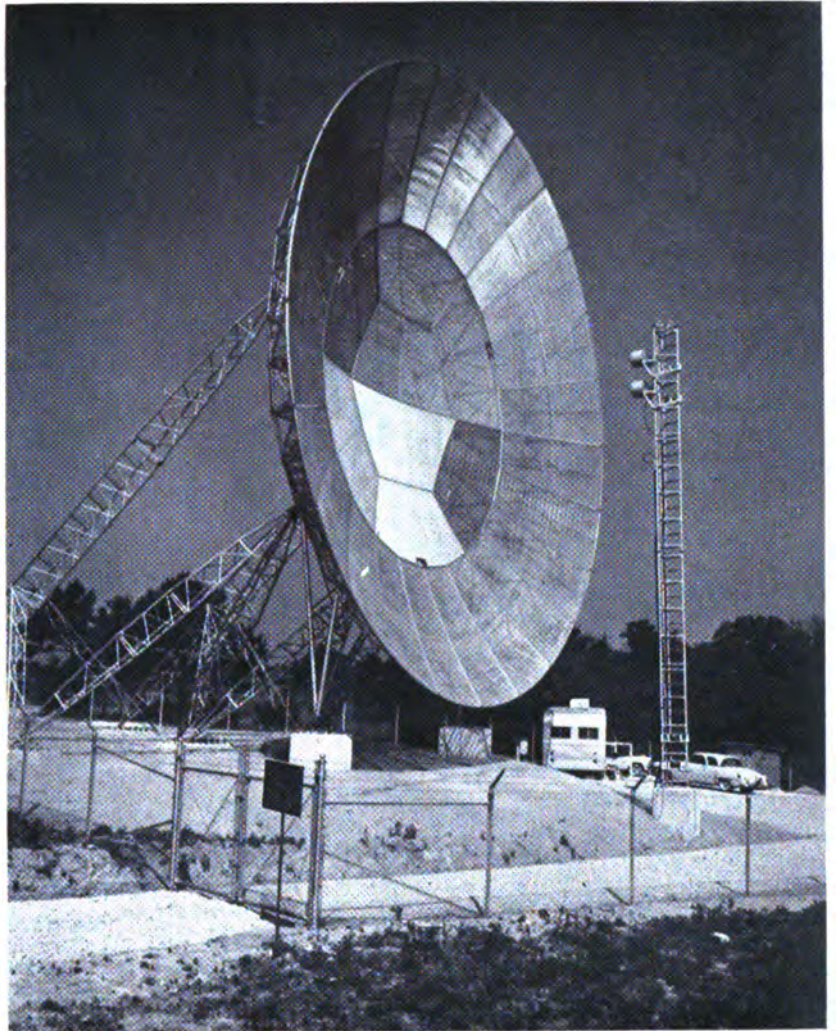
Sixty-foot paraboloidal-reflector antenna, typical of those tested and operated by PAGE for Lincoln Laboratory, M.I.T.
