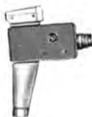
"Telemite," smallest TV camera, features newly developed RCA 1/2-inch Vidicon tube, size 1 3/8" x 2 3/8" x 4 3/4", weighs about one pound.
