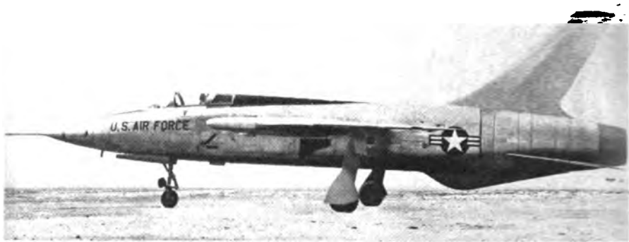
Pictured above is the Air Force's new, supersonic fighter-bomber, Republic F-105 Thunderchief, which has been selected for volume production. Flying faster than sound on its very first flight, the Thunderchief has already proved itself in more than 250 test flights. It has been designed under the Weapons System Concept as a nuclear-bomb-carrying fighter and is powered by the Pratt and Whitney J-75 engine. Outstanding design features are the long, cylindrical fuselage, the short, very thin swept-back wings, the needle nose and the ventral fin on the bottom of the aft fuselage near the tail. Scheduled to reach a production peak late in 1958, the F-105 assembly line is already in operation.
