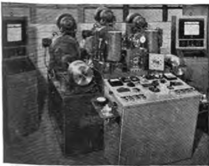
Ultra-thin tape for bobbin cores is rolled to high precision standards for thickness and finish on our own 20-high Sendzimir cold reducing mill, beta-ray controlled.
