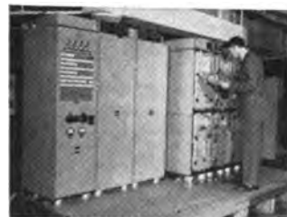
Engineer at Ford Instrument checks out computer developed and built for U. S. Navy.
