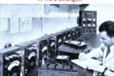
Calibration to primary standards.
