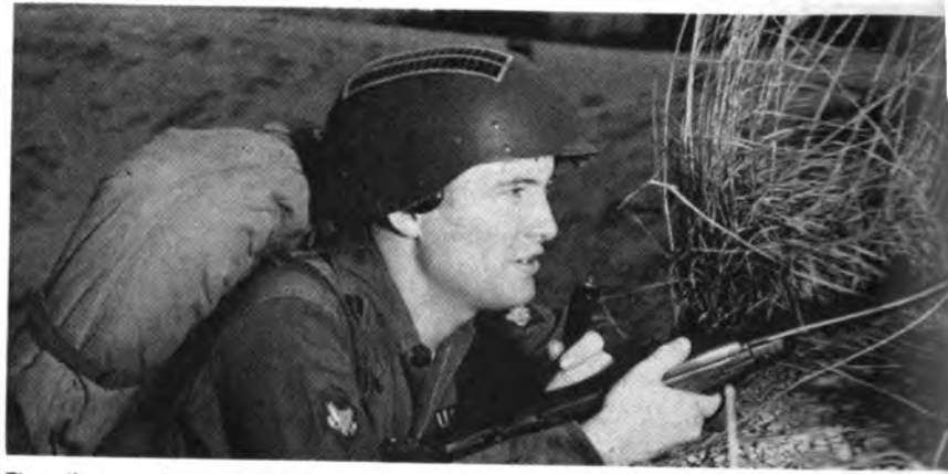
Tiny silicon wafers, or solar batteries, grouped in long narrow clusters on the crown of Army's new helmet radio, can provide all the electrical power needed to operate the transmitter-receiver. Like the original helmet radio, the sun-powered version is a development of the U. S. Army Signal Engineering Laboratories, Fort Monmouth, New Jersey. Teamed with small nickel-cadmium storage batteries for peak power and nighttime operation, the solar cells can provide current for as much as a year, as compared with dry cell life measured in hours.
