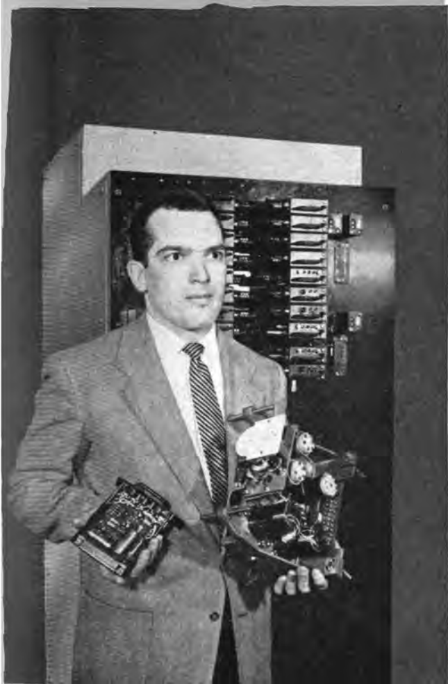
Robert Rossler, FICo engineer, holding plug-in analog modules — a transistorized amplifier unit and an electro-mechanical unit. Electronic panel of analog computer is in background.
