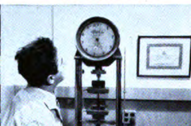
Quantitative checking of weld strength.
