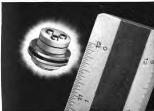
ABOVE: the GL-6917 voltage-tunable magnetron is extremely small and compact—only \frac{5}{8} " high and less than \frac{3}{4} " in diameter. BELOW: complete cavity and magnet assembly for the GL-6917 has been developed to assist equipment manufacturers.
