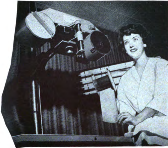
Pictured here is the film for the Micro-Master camera. It is exposed in long rolls that are automatically transported as each frame is made from one magazine to another.
