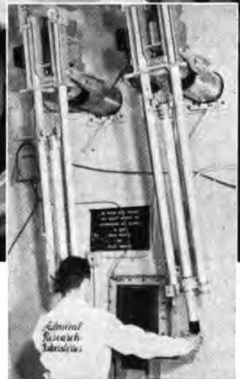
Here, in Admiral's Nucleonics Laboratory, radiation tests are conducted with a cobalt 60 source rated at 20,000 curies. The observer is shielded by 41 inch walls of magnetite ore within steel shells, and a 42 inch lead glass window.
