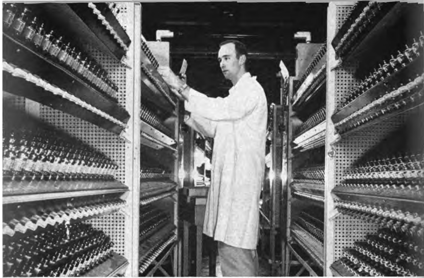
General Electric technician checks 5-Star Tubes on special 46-hour inoperative control test, designed to reduce early-life failures. His lint-free, white Nylon garb marks this process as part of Operation Snow White—General Electric's all-out program to exclude from 5-Star Tubes any impurities that can cause short circuits or impair electrical efficiency.
