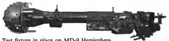
Test fixture in place on MD-9 Hemisphere Sight which we build under subcontract for the Crosley Division of Avco.
