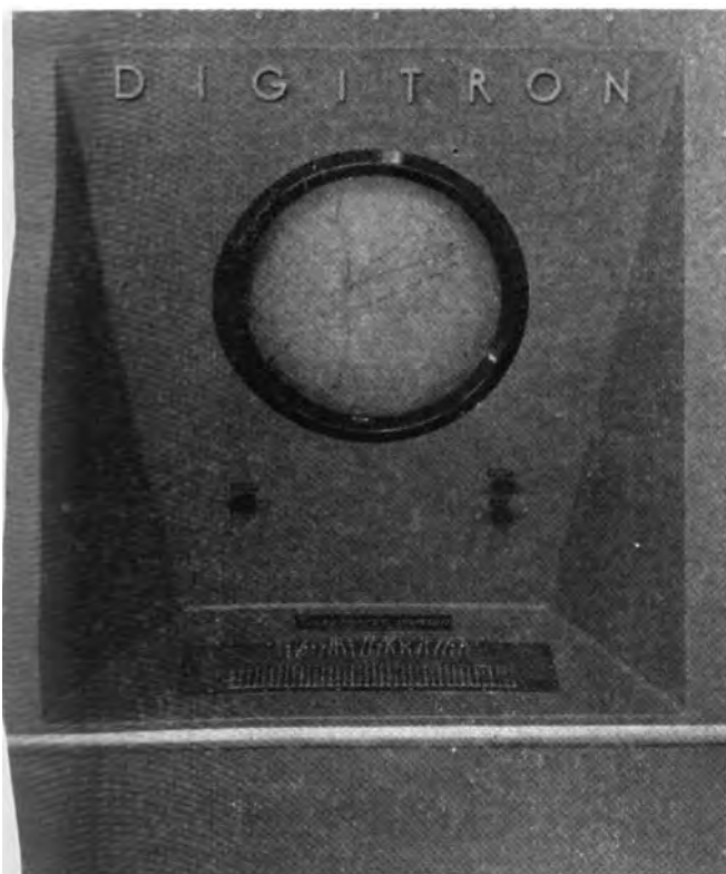
ADVANCED ELECTRONIC DATA DISPLAY EQUIPMENT exhibited by the Electronics Division of American Machine & Foundry Company, Boston, Mass., at the 1957 National Conference of the Institute of Radio Engineers. An air-traffic control display is shown on the screen. Electronic data display systems are used whenever processed electronic information is presented to a human operator. Applications include radar, air and ship traffic control, defense systems, combat information centers, and general purpose digital computer outputs. Figure 2.
