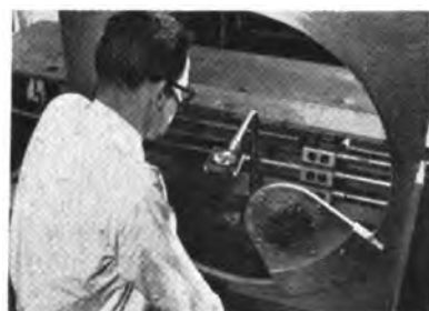
Engineer of Ford Instrument Company checking unit designed by the Company for the Air Force to be certain that its magnetic effects will not affect other instruments in the aircraft.
