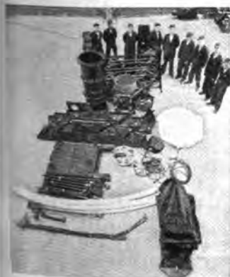
In less than one hour, this small crew can assemble the revolutionary Paraballoon antenna from these few parts. They will place the tripod directly on the ground.
