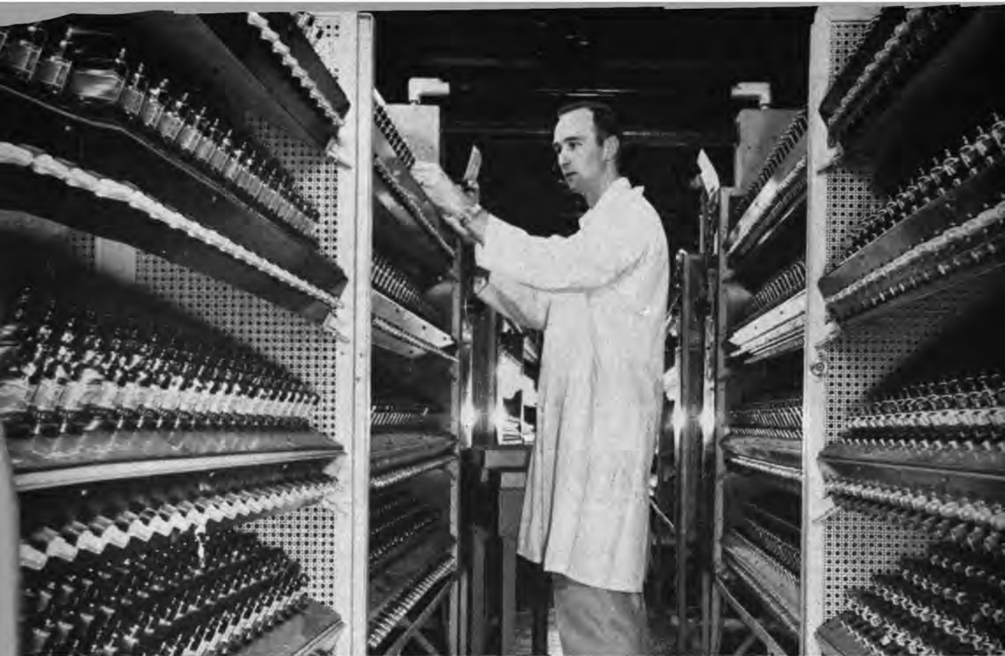
General Electric technician checks 5-Star Tubes on special 46-hour inoperative control test designed to reduce early-life failures. His lint-free, white Nylon garb marks this process as part of Operation Snow White—General Electric's all-out program to exclude from 5-Star Tubes any impurities that can cause short circuits or impair electrical efficiency.
