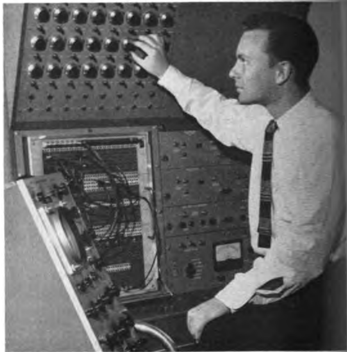
RCA Fellow studying at the New York University College of Engineering is shown verifying transistor equivalent circuits on the University's electronic analogue computer.
