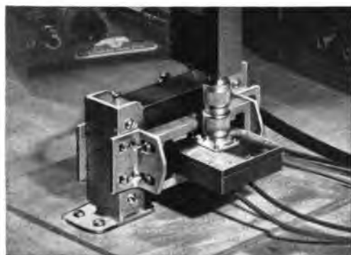
ABOVE: the GL-6917 voltage-tunable magnetron is extremely small and compact—only \frac{5}{8} " high and less than \frac{3}{4} " in diameter. BELOW: complete cavity and magnet assembly for the GL-6917 has been developed to assist equipment manufacturers.
