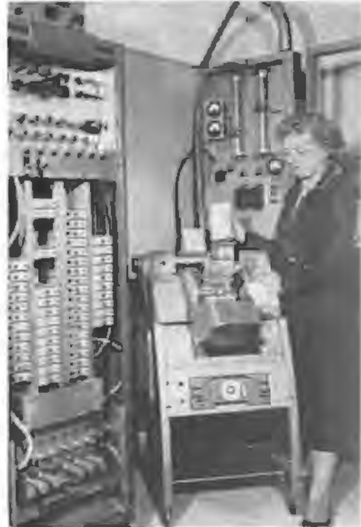
Fig. 1, left: Inscriber: punched paper tape to magnetic wire converter.
