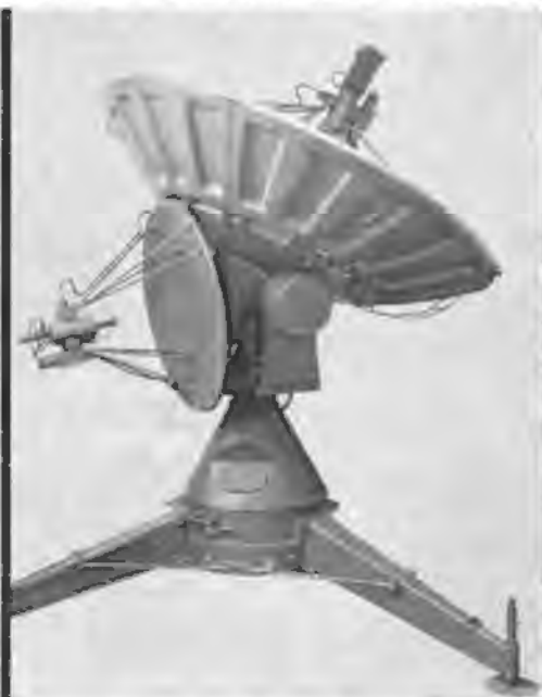
Lightweight, ground-based, air-transportable, dual reflector, multi-band, high gain search antenna and control system; 2-speed data systems and magnetic clutch drives in azimuth and elevation.
