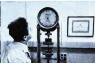
Quantitative checking of weld strength.
