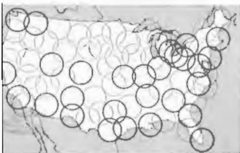
Raytheon radar at 23 of the 28 heavily circled areas will be an integral part of C.A.A. control network. Light circles indicate future coverage.
