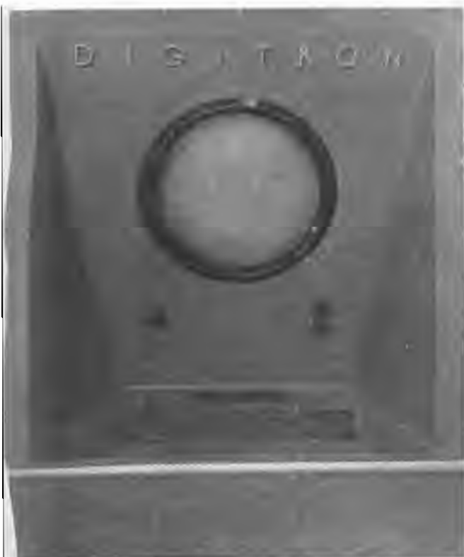
ADVANCED ELECTRONIC DATA DISPLAY EQUIPMENT exhibited by the Electronics Division of American Machine & Foundry Company, Boston, Mass., at the 1957 National Conference of the Institute of Radio Engineers. An air-traffic control display is shown on the screen. Electronic data display systems are used whenever processed electronic information is presented to a human operator. Applications include radar, air and ship traffic control, defense systems, combat information centrals, and general purpose digital computer outputs. Figure 2.
