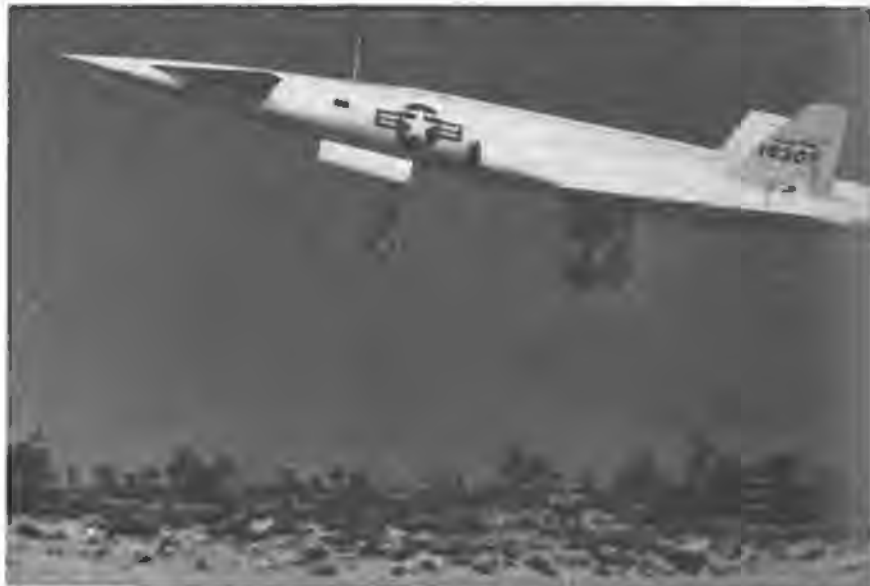
Pictured above is North American Aviation's new X-10, an unmanned test vehicle for the Air Force SM-64 NAVAHO inter-continental strategic guided missile program, which has been recently tested in flight at the USAF Missile Test Center, Florida. Called "an invaluable source of important data," the X-10 is powered by two turbo-jet engines and is provided with a landing gear so that it can be recovered for repeated use. Design and manufacture of the NAVAHO guidance and control systems is the responsibility of North American's Automatics Division, and a third division, Rocketdyne, is building rocket engines for the missile, which will be rocket-boosted to flying speed and then powered by ram-jet engines. The NAVAHO will travel at supersonic speeds and very high altitudes, with great accuracy of delivery.
