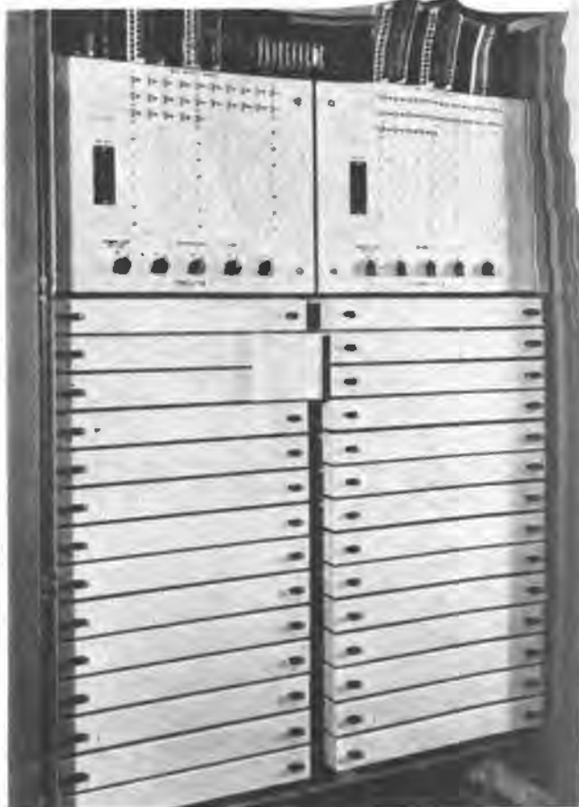
Translator, front view, converts message to proper circuit
