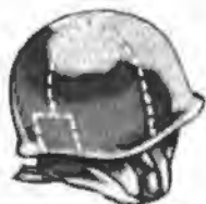
Transistorized radio receiver transmitter completely concealed in helmet has up to 5-mile range.
