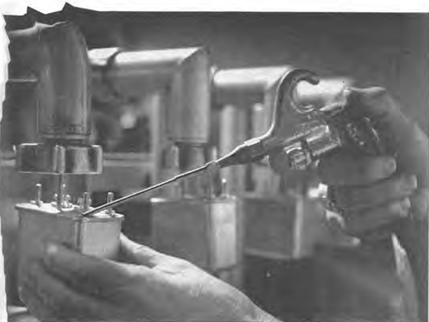
Tracer gas is sprayed over the relay enclosure while it is under high vacuum
