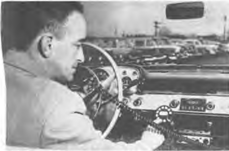
Simple dialing procedure for using automatic "dial-direct" mobile two-way radiotelephone system, developed by Du Mont, is here demonstrated by engineer James A. Craig.
