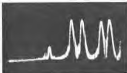
Scope pattern taken from Hoffman CV-157 showing two dualtone teletype channels on upper sideband, carrier partially suppressed. Each sideband can carry 32 teletype channels at one time.
