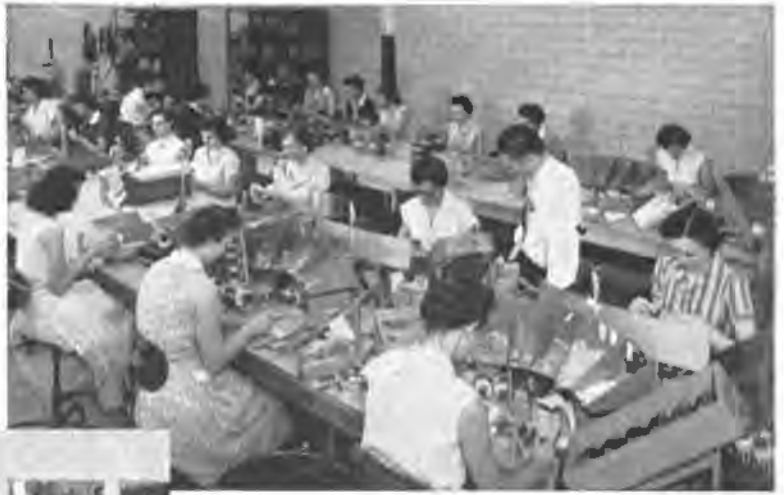
Photo at right shows operators inserting secondary coils and connecting leads to commutators for units like the compact Sangamo "GY" Flatpak—a rugged, small size dynamotor for mobile radio use.
