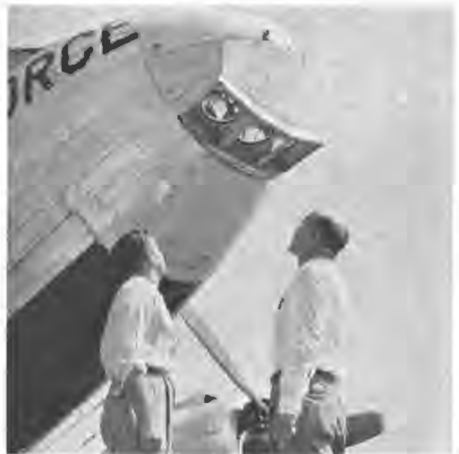
These three, small lights mounted in the nose of a C-47 test aircraft provide sufficient, continuous light for night aerial photography.
