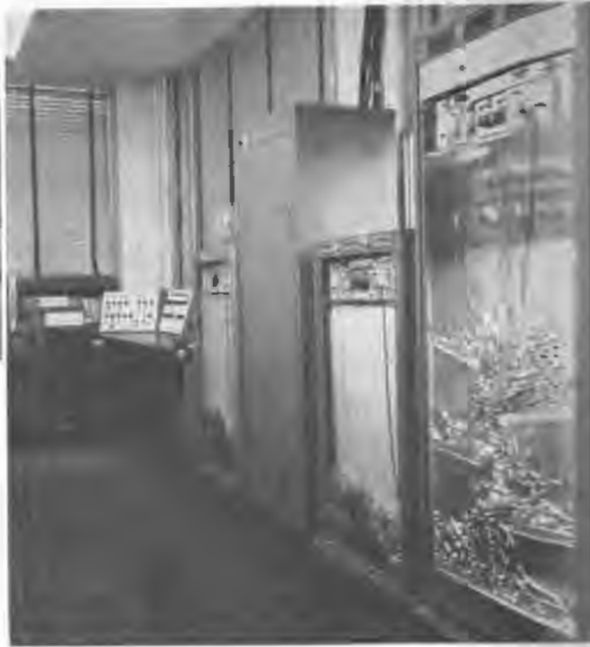
Both single-channel and multi-channel tape drive mechanisms have been added as an auxiliary memory.
