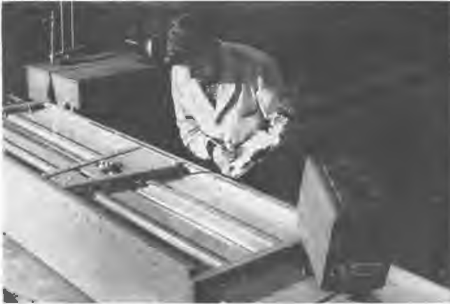
The Slotted Line for Wave Guides, manufactured by I-T-E Circuit Breaker Co., Philadelphia, Pa., fills a need in the fields of radar and scatter communications. Instruments similar to the one pictured above currently are being supplied for both military and commercial installations.
