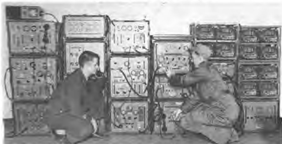
Assembled above is terminal equipment, telephone AN/TCC-7 and radio terminal set AN/TRC-35
