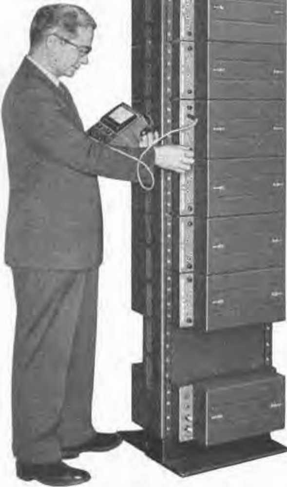
To change channel assignment, simply change one plug-in crystal.
