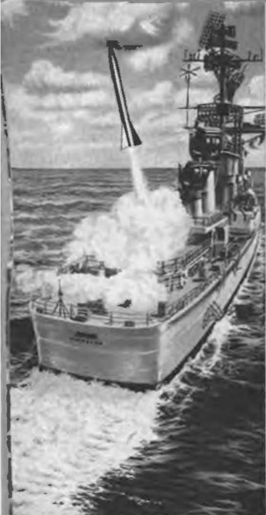
MISSILE CRUISER —Problem: To launch a missile 1500 miles from target. An error of only 1 degree in launching information would cause a 25-mile target miss.
