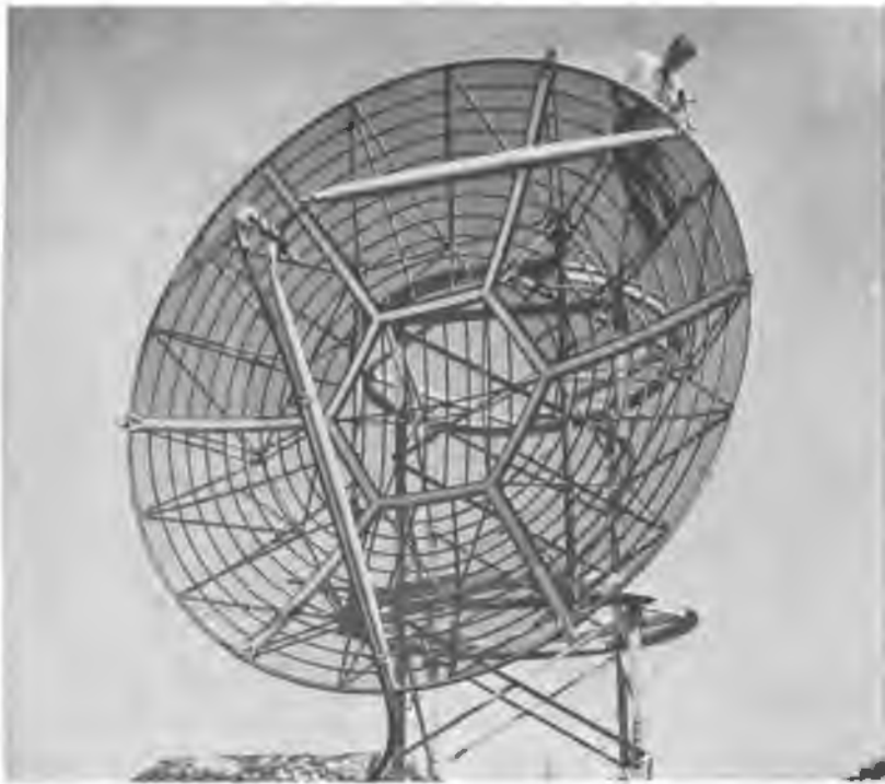
A senior Engineering Assistant of Western Union's Radio Transmission Division adjusts large "forward scatter" microwave antenna atop the telegraph company's building in New York City. The antenna is used for beyond-line-of-sight tropospheric radio signal propagation tests between New York and Philadelphia.
