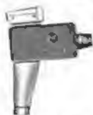
"Telemite," smallest TV camera, features newly developed RCA 1/4-inch Vidicon tube, size 1 1/8" x 2 3/8" x 4 3/4", weighs about one pound.
