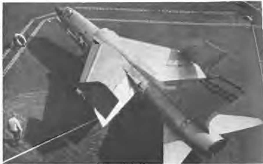
FBU about to taxi off elevator and onto catapult of CVA-59 during carrier suitability trial.
