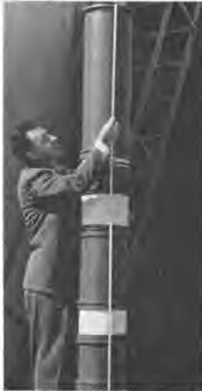
The world's largest electron tube—a ten-foot five-inch klystron—is measured by W. W. Eitel, president of Eitel-McCullough, Inc., manufacturers of Eimac electron tubes. The new giant super power tube will be used in radar and linear accelerator applications.
