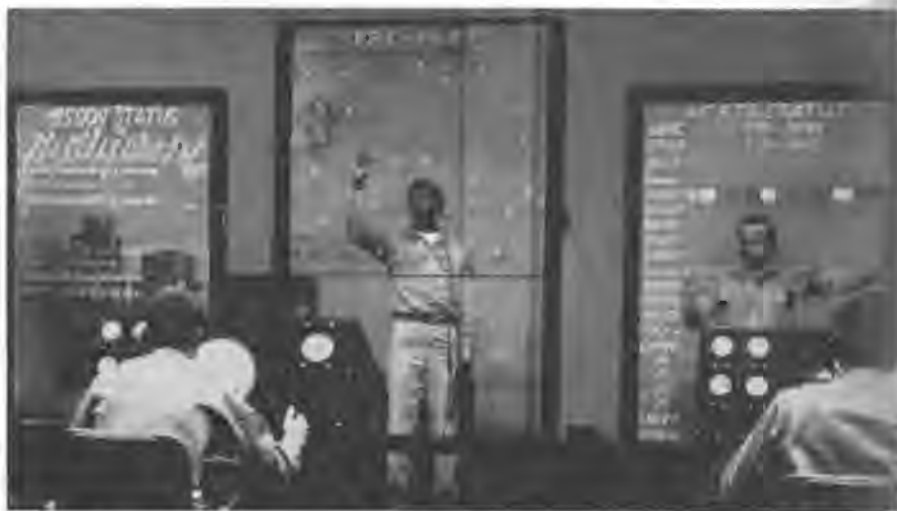
Displayed above is the operation of the new ground intercept system. Developed by G-E, it receives signals from radars within the Air Defense Command, computes them and directs our interceptors to the proper position to destroy potential bombers. These signals are automatically incorporated into the fire control system rather than being sent as a verbal command as has been previously done.
