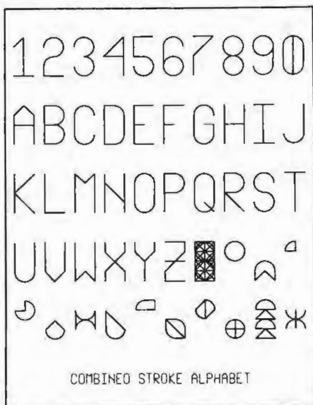
A possible form of symbology available in the DIGITRON display equipment developed by the Electronics Division of American Machine & Foundry Company. Figure 3.
