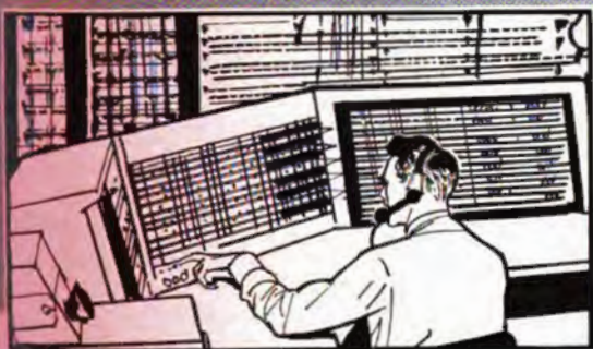
Sage "Brain". Giant electronic computers receive and store defense data . . . furnish correct picture to commanders at earliest possible moment.
