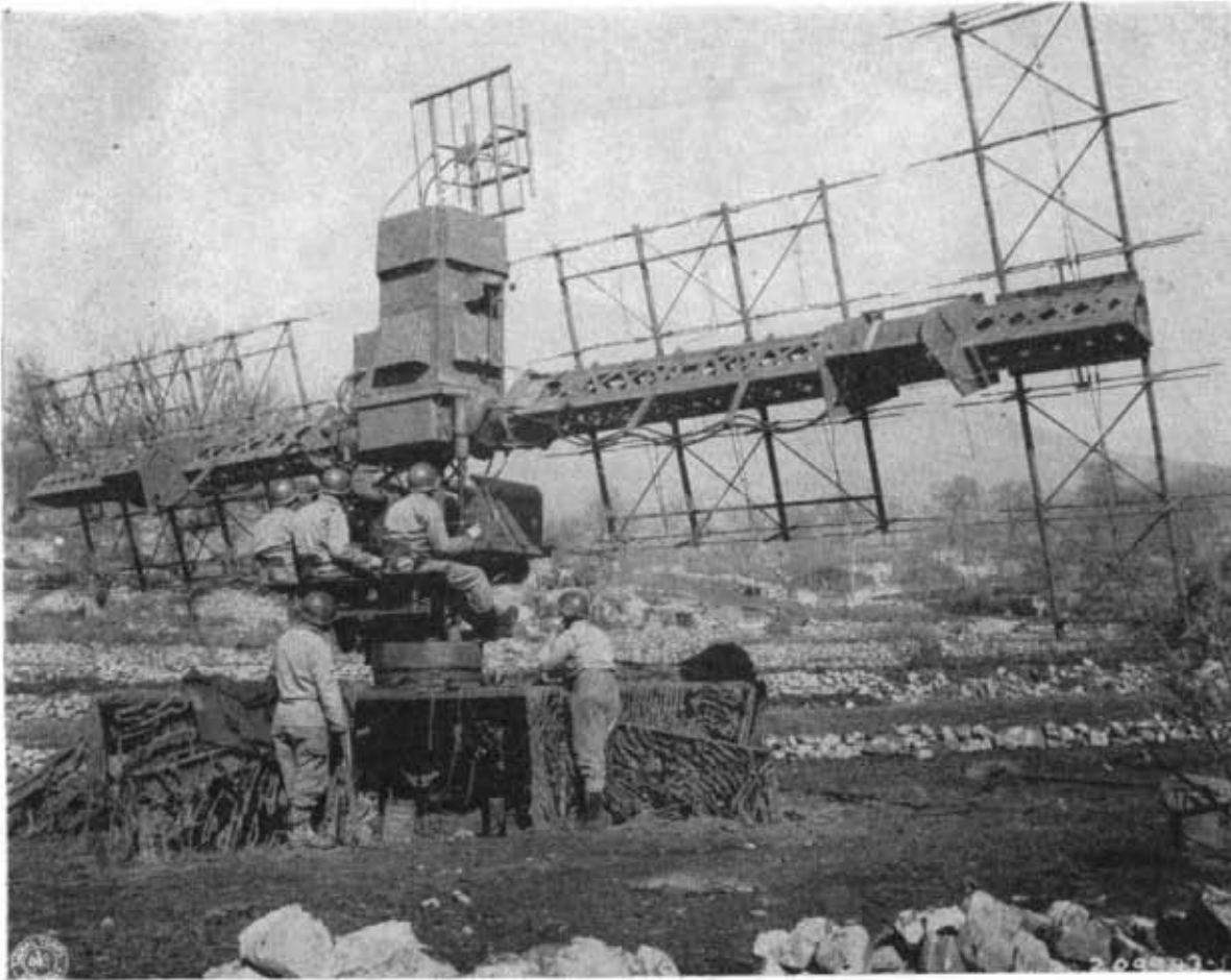
Radar in operation: Radio set SCR-268 with a five man crew is shown in operation on an Italian hillside. The three operators seated on the mount see indications of the airplane echo on cathode ray oscilloscopes. One operator tracks the aircraft in azimuth; another operator tracks in elevation and the third measures the range.
