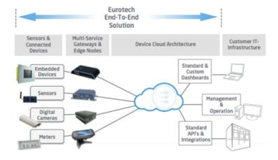
One of he most important aspects of the "Internet of Things" (IoT) vision is that smart objects communicate effectively with each o her and with applications residing in data centers or the cloud. Eurotech develops and offers the technical building blocks required to build distributed systems of devices and sensors to be effectively interconnected with IT infrastructures
