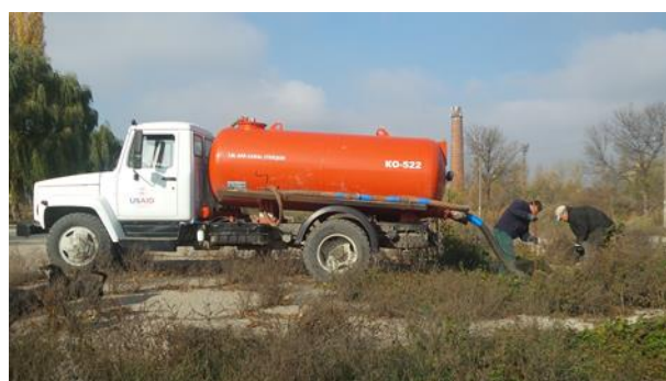
A donated sewer cleaner truck at work in Straseni.
